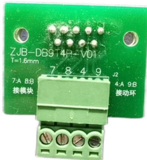
Fig7 Supporting adapter board for touch screen
